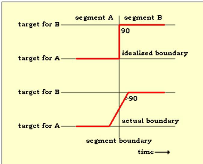
Fig. 4 Comparison of idealized and real boundary transitions.
