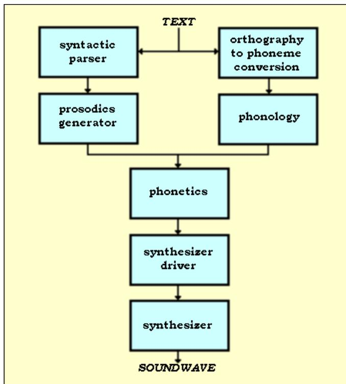
Fig. 2 A typical text-to-speech synthesis system.
