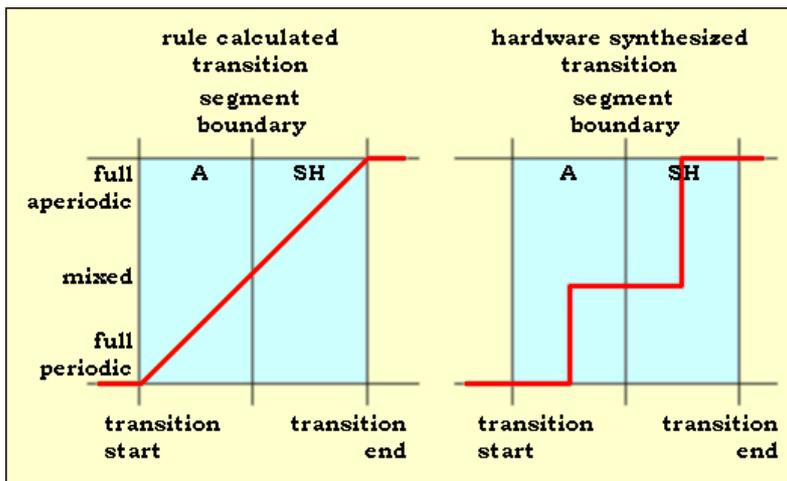
Fig. 5 Voicing parameter transition, showing hardware distortion (on the right) of the calculated transition between full periodic excitation and full aperiodic excitation.
