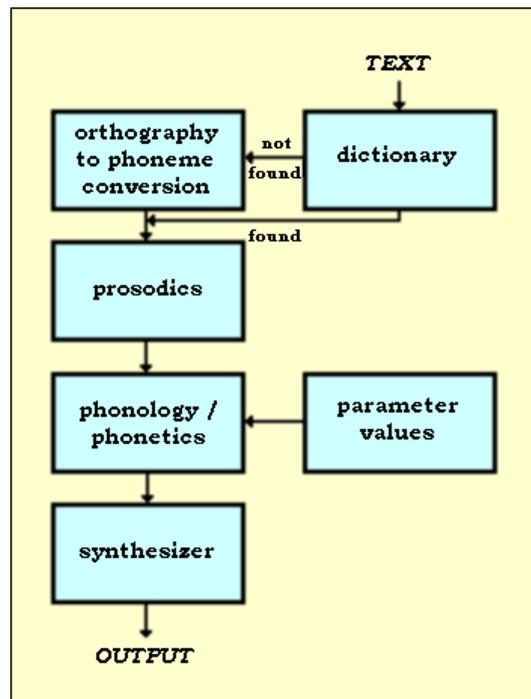
Fig .1. Text-to-speech synthesis system.
