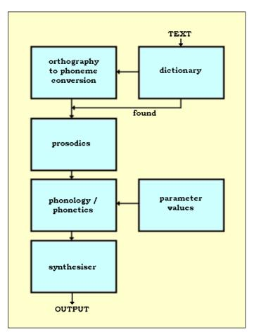
Fig. 22-2. Linguistic levels of description as components of a standard synthesis algorithm
