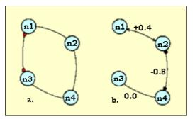
Fig. 1. Generalised network, showing four types of connection with numerically specified thresholds. A simple, unterminated edge represents an unspecified connection; an arrow terminated edge an excited connection; a black circle terminated edge an inhibited connection; a red circle terminated edge an impossible connection.
