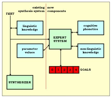
Fig. 2. Block diagram of the general system architecture.
