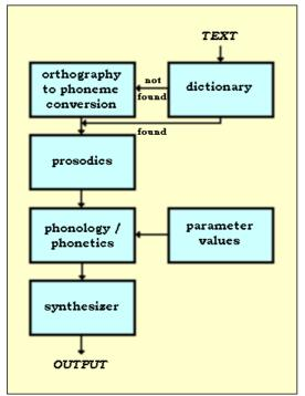
Fig .1. Text-to-speech synthesis system.
